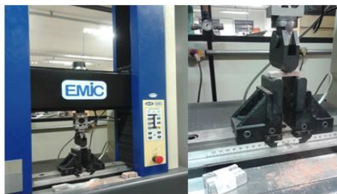
Fig. 6. Bending test in test specimen
