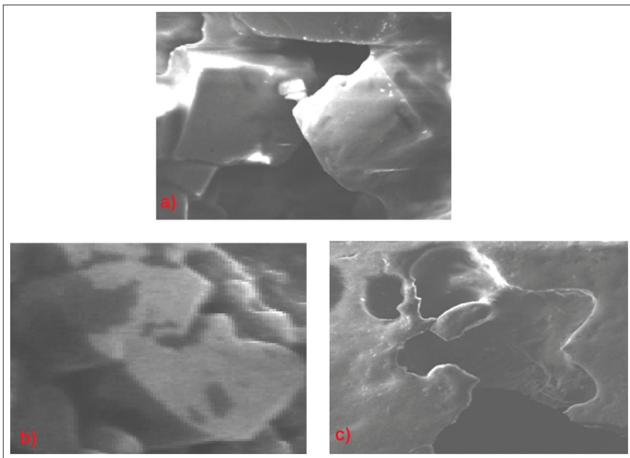
**Figure 4.** SEM images of NHC complexes, compounds (a) 3a, (b) 3b and (c) 3c. Inset: Time of sample gathering (days) (a) 500  $\mu\text{m}$ , (b) 300  $\mu\text{m}$  and (c) 500  $\mu\text{m}$  scale bar.
