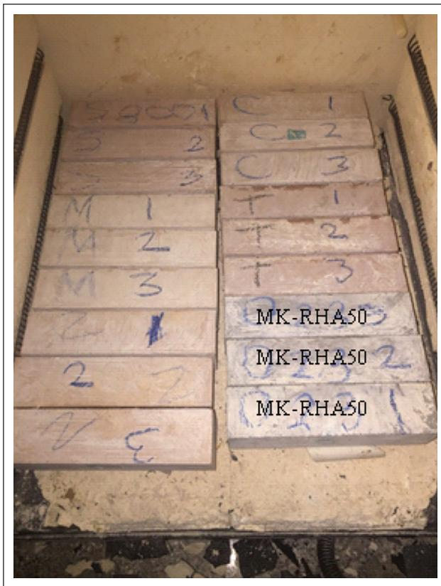
**Figure 6.** The prism specimens placed in the furnace.
