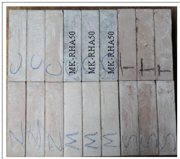
**Figure 2.** The prism specimens after curing.
