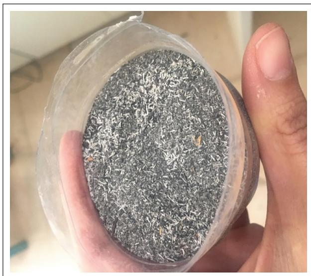
**Figure 1.** Burned rice husk ( $\geq 63 \mu\text{m}$ ).
