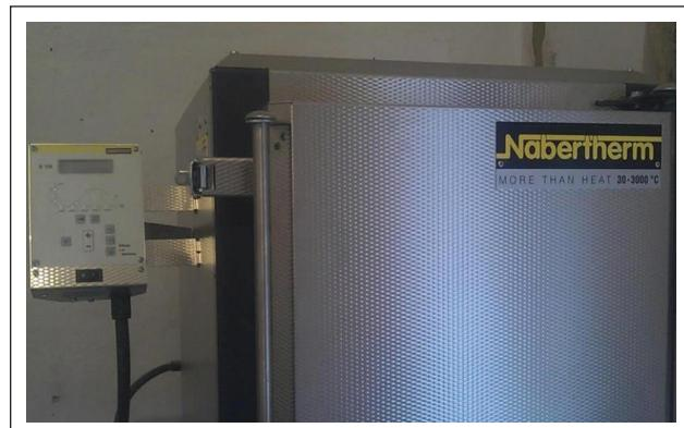
**Figure 5.** Nabertherm B130 high temperature electric furnace.
