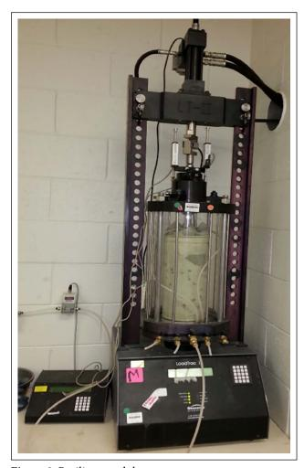
Figure 2. Resilient modulus test setup.
