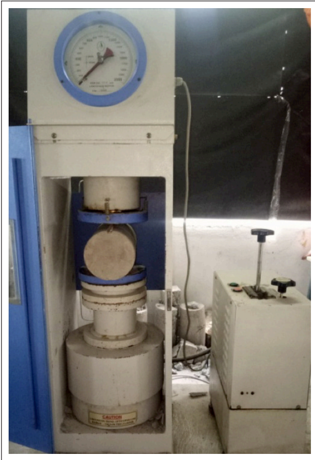
Figure 6. Experimental photograph of Split tensile strength test.
