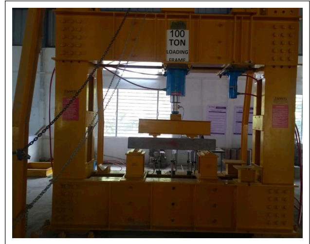
Figure 7. Experimental photograph of Flexural strength test.
