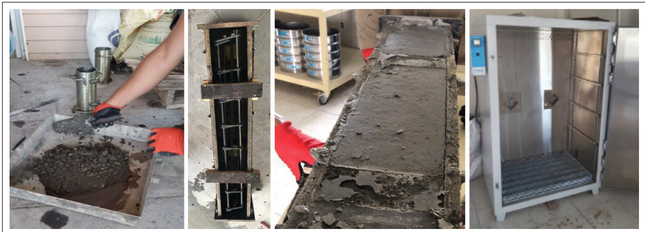
Figure 2. Placing and curing concrete in molds.
