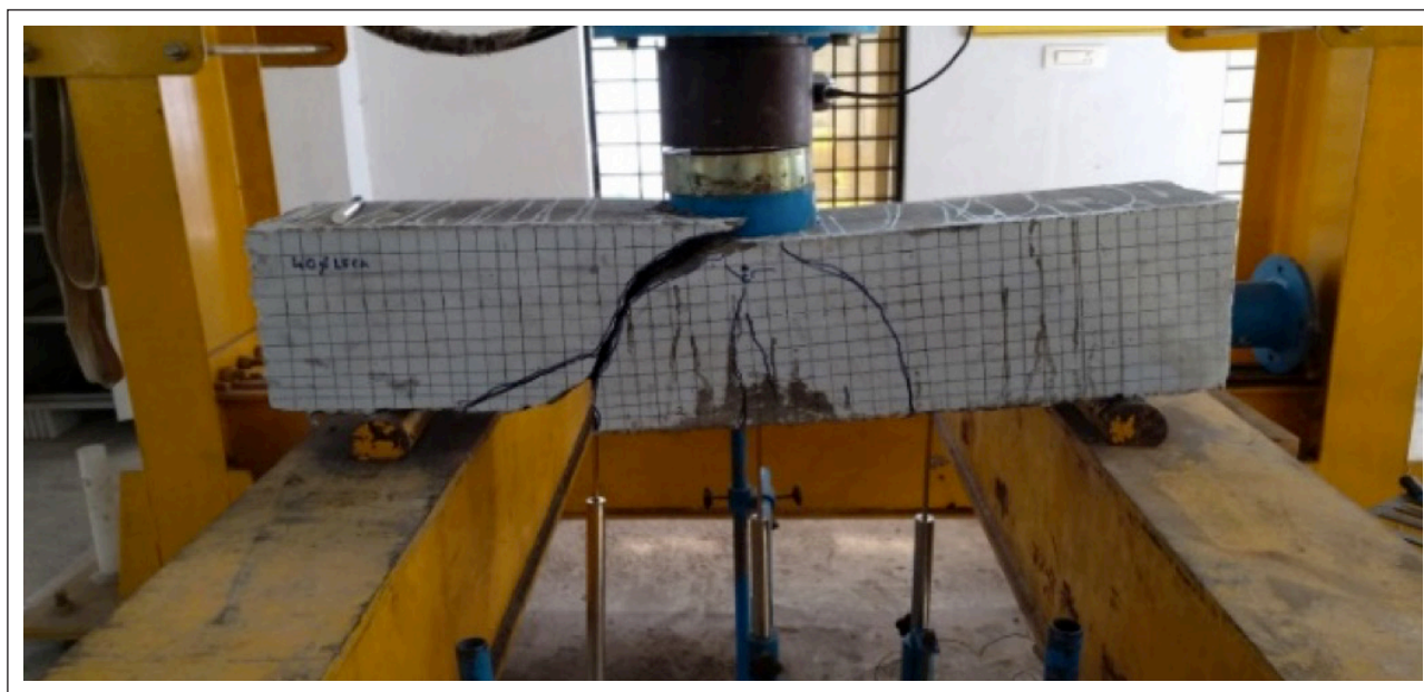
Figure 11. Crack pattern of beam LECA 20.
