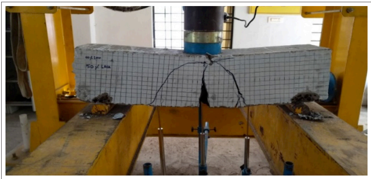
Figure 12. Crack pattern of beam LECA 25.
