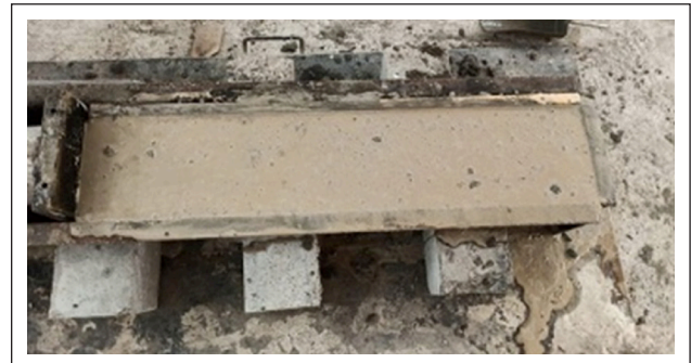
Figure 2. Mould with casted beam specimen.
