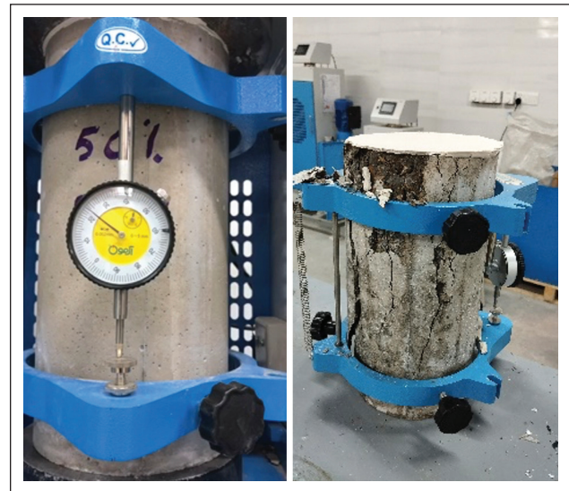
Figure 5. Measuring the stress-strain curve (left image is before testing, right image is after testing).
