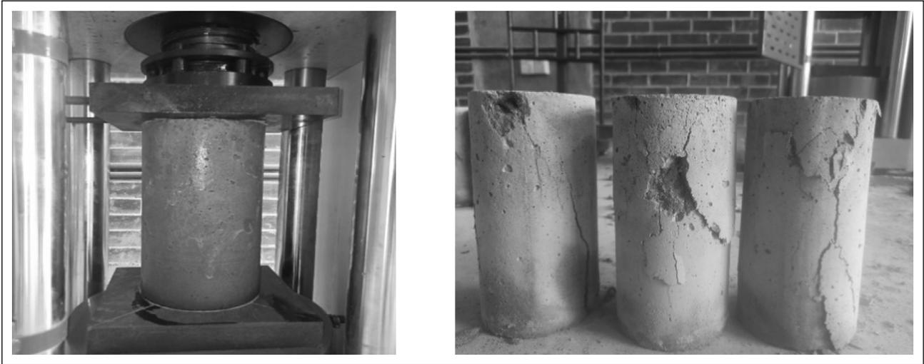
**Figure 5.** Applying the load to the cylinder specimen to measure its load-bearing capacity.
