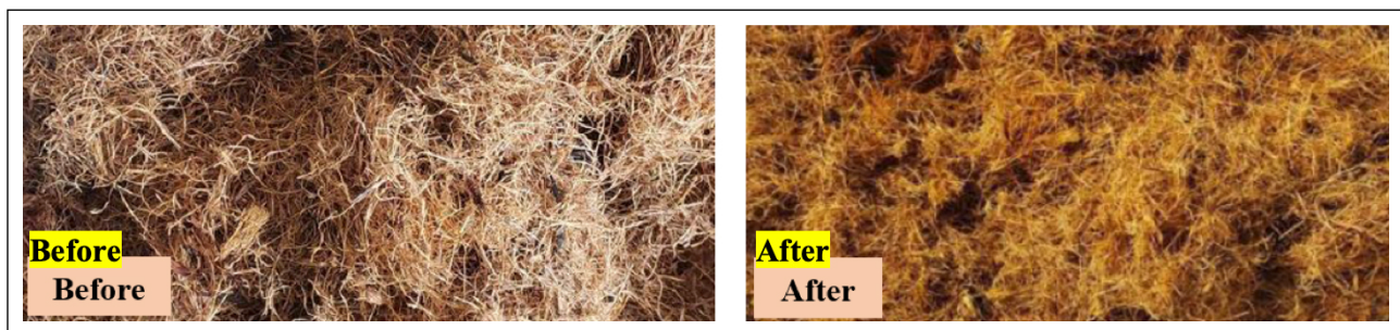
Figure 5. PFBF used in the study: Before and after hot water and alkali treatment.
