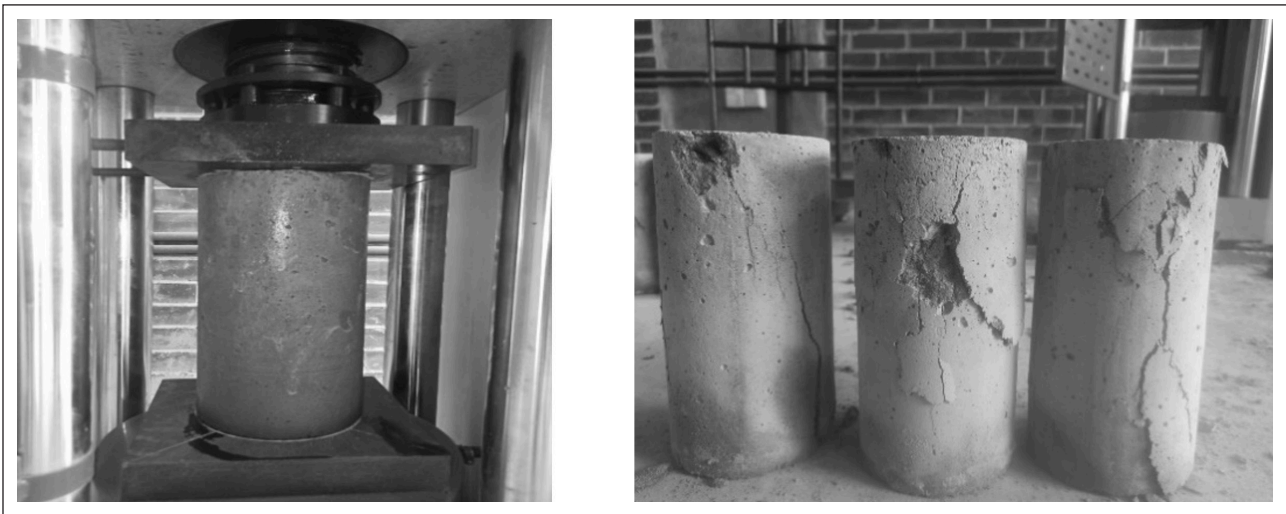
Figure 5. Applying the load to the cylinder specimen to measure its load-bearing capacity.
