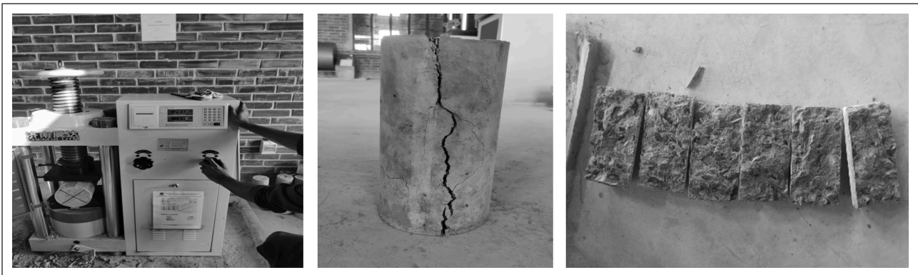
Figure 6. Application of load to the cylindrical specimen to evaluate the split tensile strength and the specimen's failure behavior.
