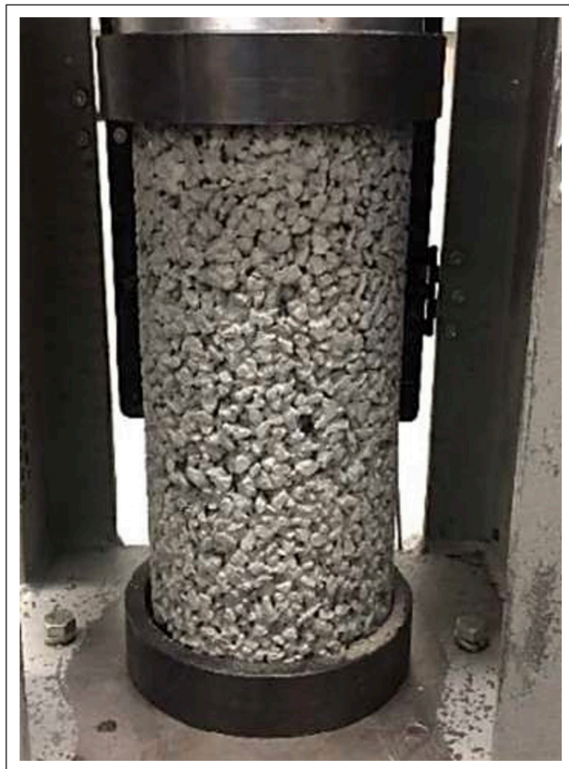
Figure 5. As per ASTM C39, the compressive strength test.
