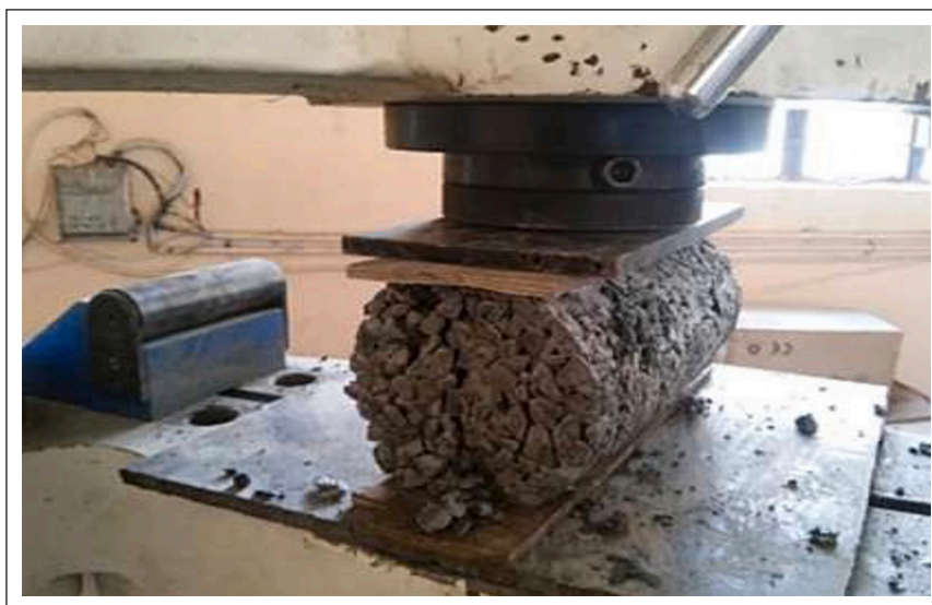
Figure 9. Tensile strength determination using the Brazilian approach.
