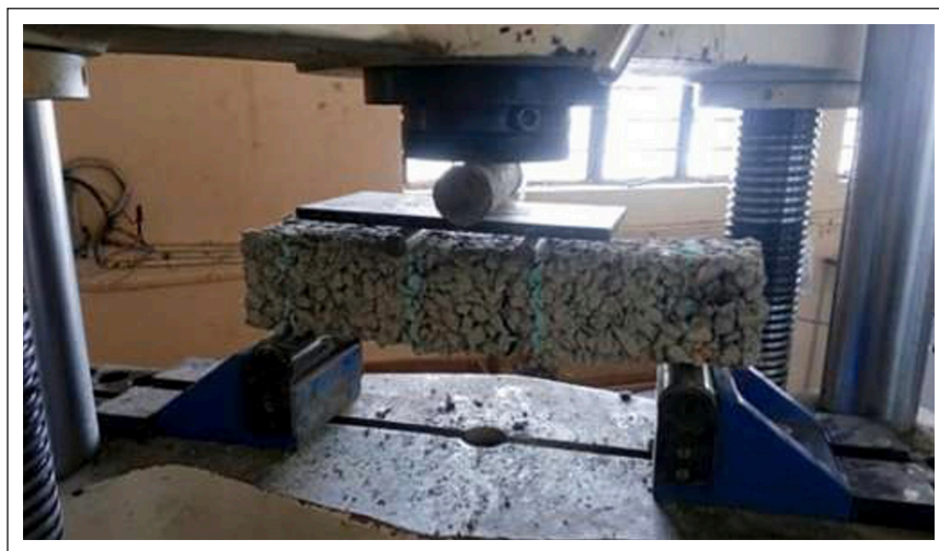
Figure 8. Flexural strength testing following the ASTM C78 standard.
